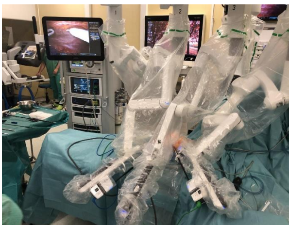
Figure 4. Docked robot at ports
